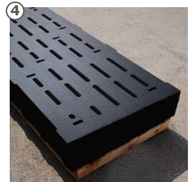
based on the CAD created drawing, the slits are cut exactly into the mats with innovative water jet technology
