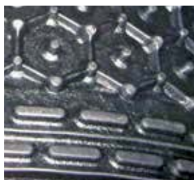
sealing lips on lower side
