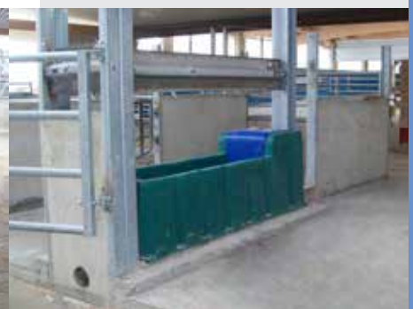
Option I: 1x MAXIFLOW float valve (connected to a feed pipe, shown with a frost protection heating cable 24 V, 20 W, 2 m), 1x heating element 24 V, 180 W
